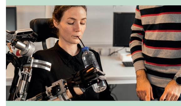
The EXOTIC exoskeleton developed at the Centre for Rehabilitation Robotics is the world's first tongue-controlled full arm/hand exoskeleton to empower individuals who are completely paralysed from the neck down to drink and eat on their own.
