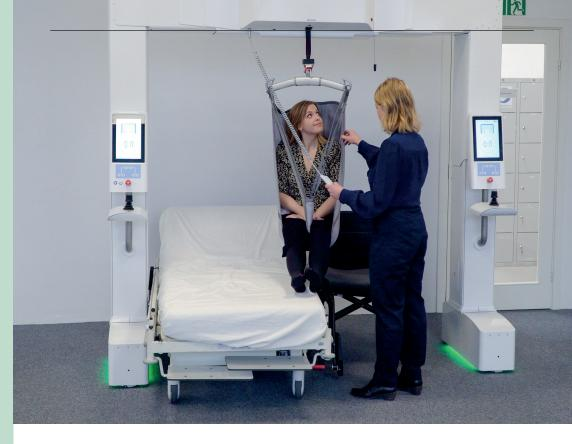
Wishing to create a flexible tool for more efficient work routines and a safer working environment, Zealand University Hospital Køge and Blue Ocean Robotics joined forces in developing the PTR robot. Offloading the heavy lifting by handling patients up to 250 kg (550 lbs), it frees up healthcare workers' time for responsive patient care.
