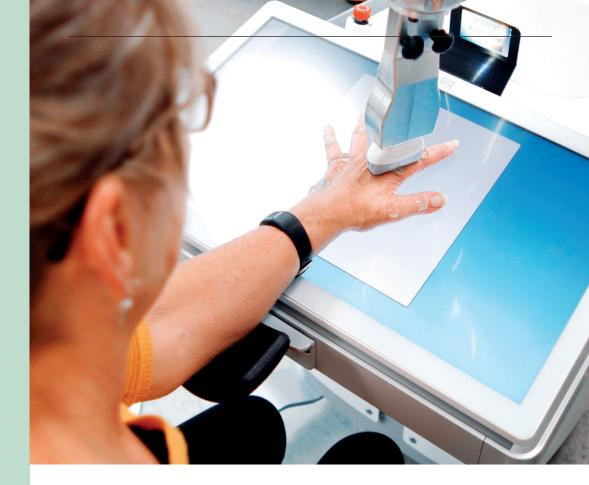
The robot's user-friendly graphical interface guides the patient from ID registration to placing their hand on the touchscreen display to performing the ultrasound scanning as the robot moves the ultrasound probe from one finger joint to the next. Each ultrasound image is scored using an AI algorithm that evaluates disease activity.
